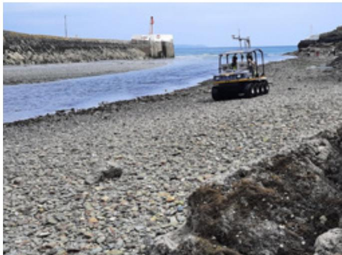
At the same time more detailed work is being carried out for the outline design of the scheme. During the summer surveyors from the MWJV design team used a small amphibious vehicle to carry out a detailed laser scan and sonar survey of the Harbour, Banjo Pier and Seawall.
